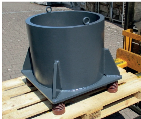
Fig. 10b: Coated chamber post welding and brushing
